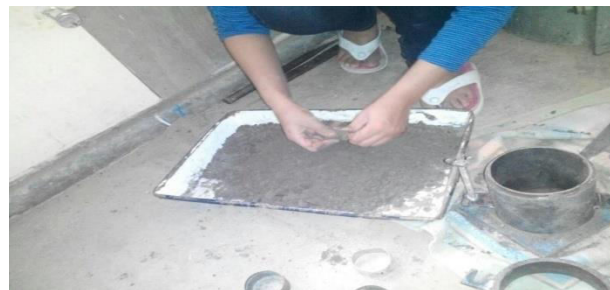
Figure Sample preparation for proctor test
