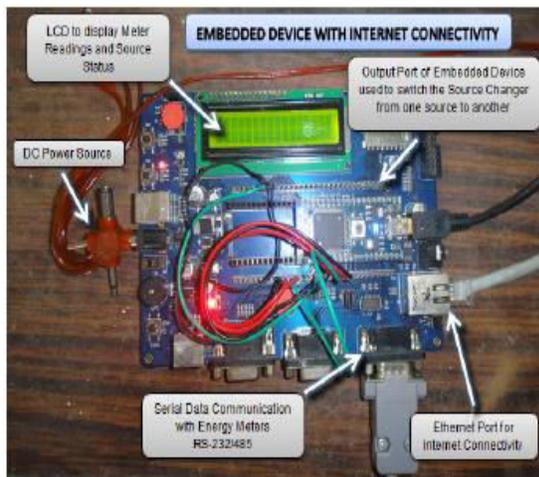
Fig2. ARM Processor based Internet Enabled Embedded Device
