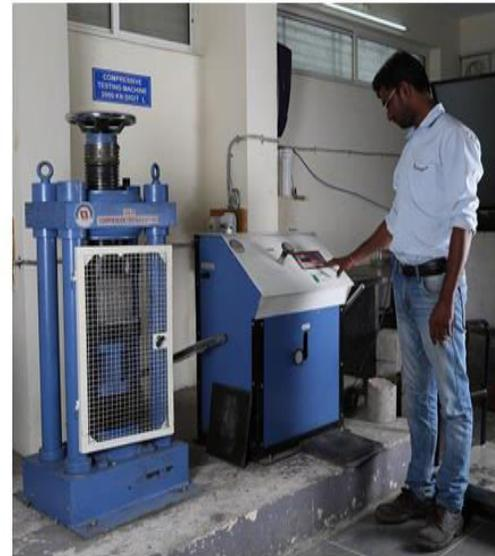
Figure shows the compression test of specimen of 150mm cube
