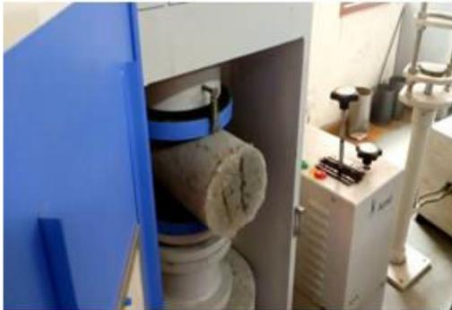
Figure shows the split tensile test
