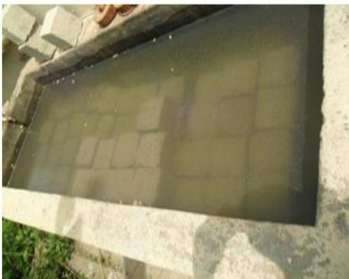
Figure shows the testing samples for curing purpose after 24 hours to dip in
