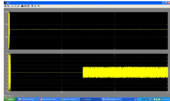
Fig.3.(a) DC link voltage. (b) Current through Capacitor.
