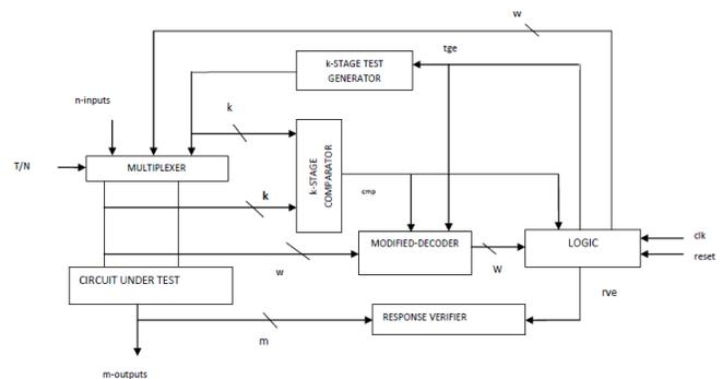
**Fig.2: SRAM based concurrent input vector monitoring BIST**
