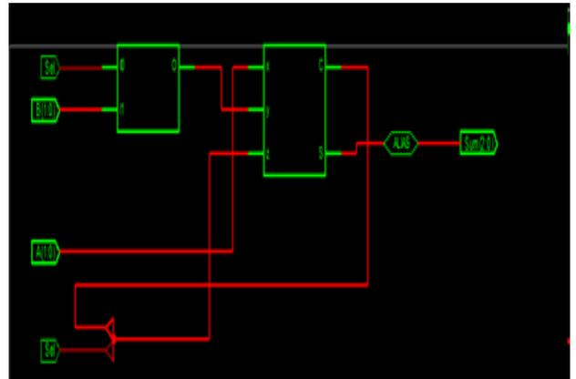
**Fig.7: RTL schematic of clock gating of modified circuit.**
