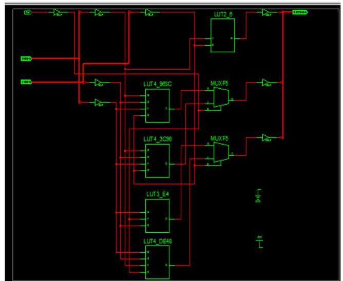
**Fig.8: Technology diagram of clock gating of modified circuit**
