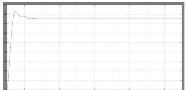
Fig.12 shows the output voltage of conventional high step-up interleaved converter
