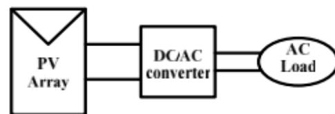
Fig.4. Block diagram representation of Photovoltaic system
