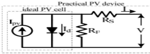
Fig.5. Practical PV device
