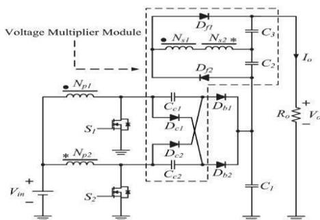
Fig. 2 Proposed high step-up converter
