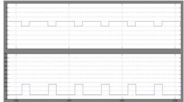
Fig.9 power switch S2 gating pulse and output voltage
