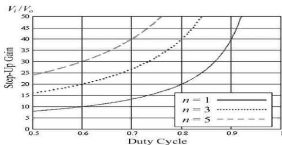
Fig. 3. Voltage gain versus turn ratio  $n$  and duty cycle
