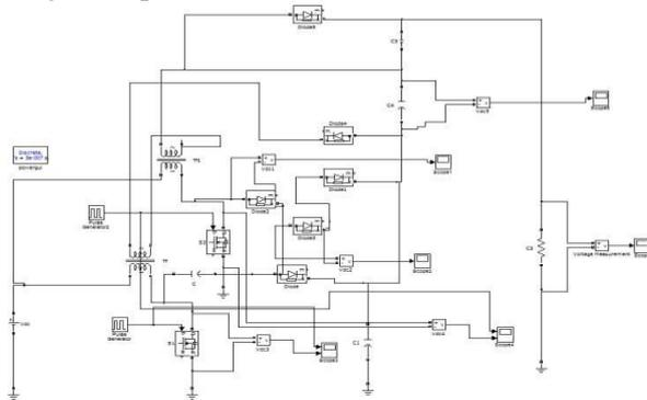
Fig.7 Simulink model of conventional high step-up interleaved converter with a voltage multiplier module
