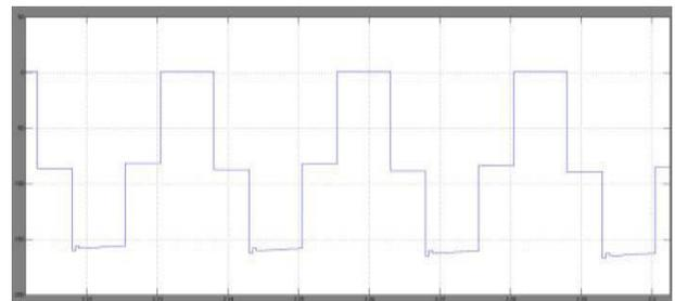
Fig.10 shows the simulated output waveform voltage across switched capacitor
