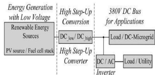
Fig .1: Block diagram of the whole system
