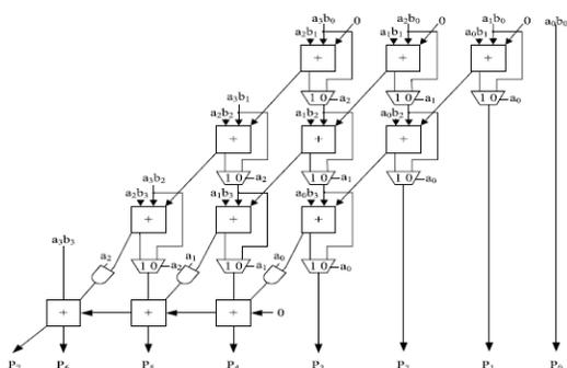
Fig 1 column-bypassing multiplier.
