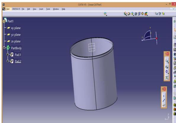
Fig.7: Sketching Cylinder model in Catia
