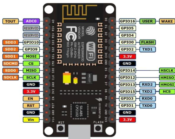
While writing GPIO code on NodeMCU, you can't address them with actual GPIO Pin Numbers as shown in Fig.4. There are different I/O Index numbers assigned to each GPIO Pin which is used for GPIO Pin addressing. Refer following table to check I/O Index of NodeMCU GPIO Pins – GPIO
