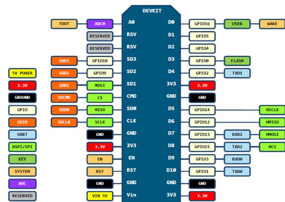
00(GPIO16) can only be used as gpio read/write, no interrupt supported, no pwm/12c/i2c supported.
