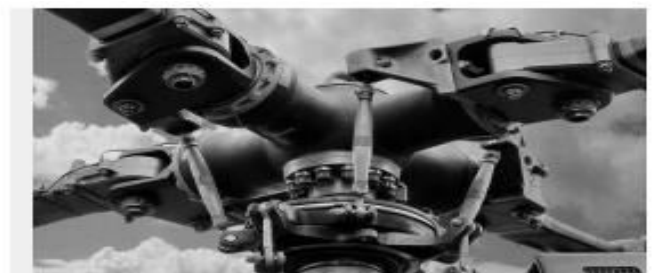
Fig. 1: Helicopter rotor system
