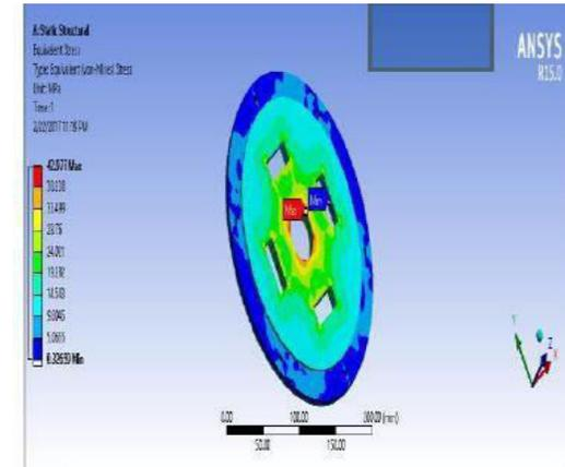
Figure 4.7 Equivalent (Vonmises) Stress
