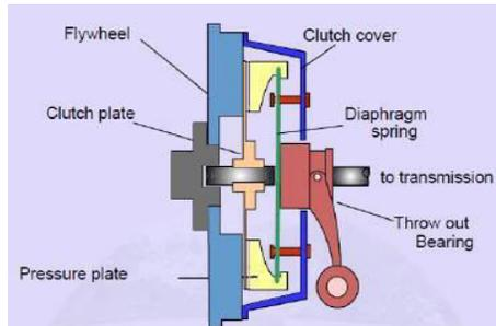
Figure 1.1 single plate clutch
