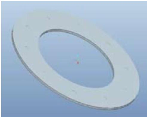
Figure 3.1 Clutch Plate
