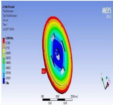
Figure 4.3 Total Deformation
