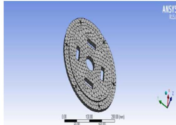
Figure 3.3 meshing of single plate clutch
