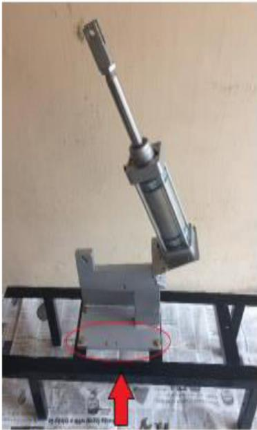
**Fig 12: Structure onto Base frame mounting**
