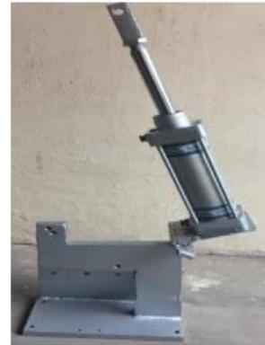
Fig 10: Support Structure with Piston Assembly
