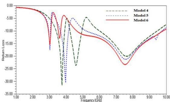
Fig. 2.2 Return Loss for Double Notch
