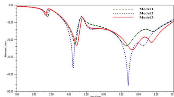
Fig. 2.1 Return Loss for Single Notch
