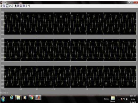
Fig5. 3-phase voltages of dual inverter fed line.
