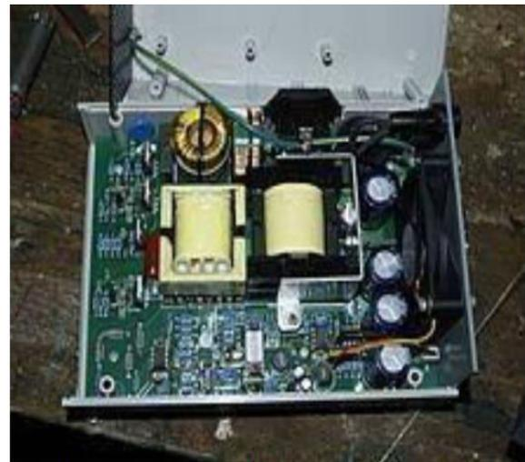
Fig2. Inside of a SWEA 250W Transformer-based grid-tie inverter.
