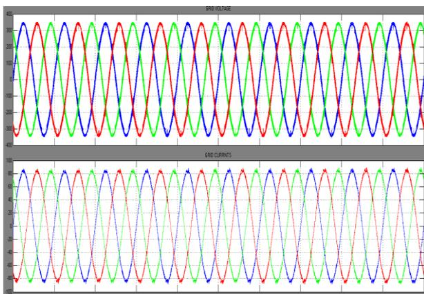
Fig.7 simulation results for grid side voltages and currents
