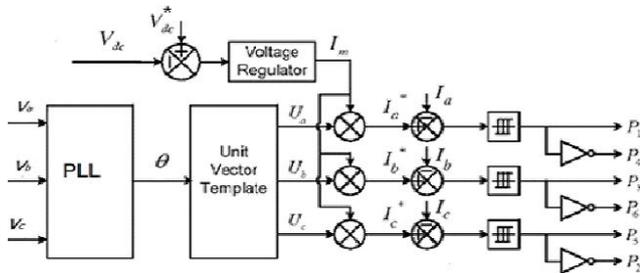
Fig. 2. Block diagram representation of grid-interfacing inverter control.
