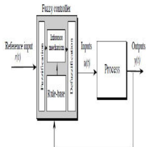
Fig.4. General Structure of the fuzzy logic controller on closed-loop system
