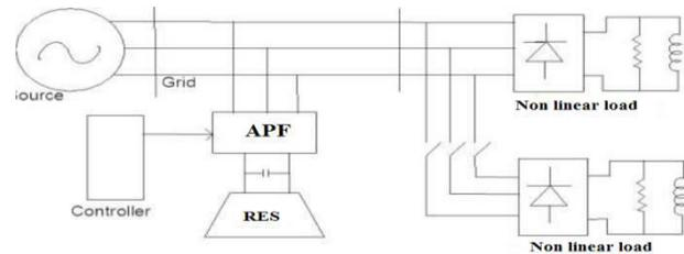
Fig 1.Schematic of the 3 phase grid system interface with renewable energy source using APF
