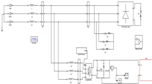
Fig.6 Matlab/Simulink of Proposed Statcom-Power Circuit
