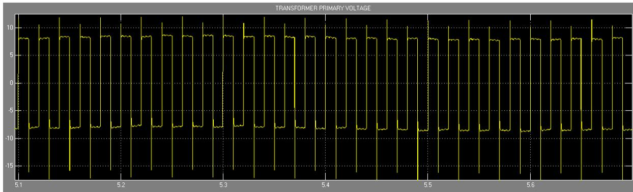
**Fig 4.Transformer primary voltage**
