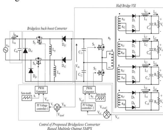
Fig.1. Proposed bridgeless-converter-based multiple-output SMPS.
