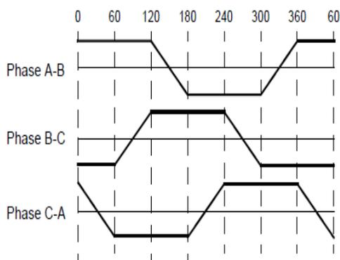
Fig.5 shows the back emf shape of the motor
