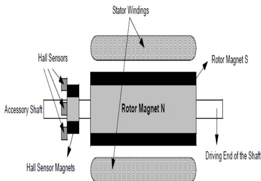
Fig.4 shows the block diagram of BLDC Motor
