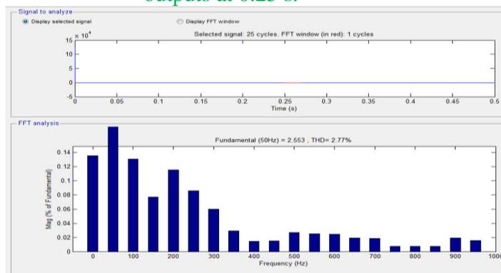
Fig 9 simulation waveform of input current and its harmonic spectrum at 220 V and full load.
