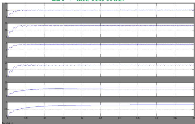
Fig 8 simulation wave form of Input voltage, current, bridgeless buck boost converter output voltage, half-bridge VSI output voltages, and currents at load variation in +12- and +5-V outputs at 0.25 s.
