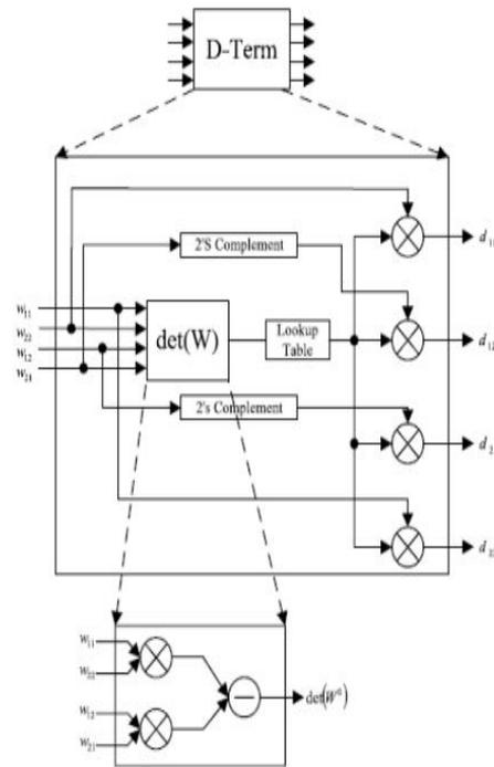
FIG 4: Architecture of a D-term unit
