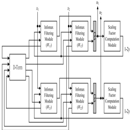
FIG 1: The block diagram of a proposed CBSS system
