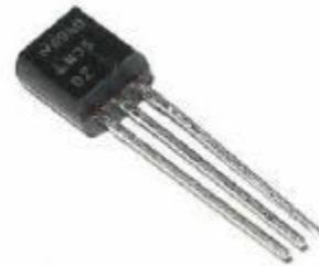
Fig 3. Temperature Sensor LM35
