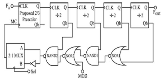
Fig.3.2. Block diagram of 32/33 and 47/48 modes.
