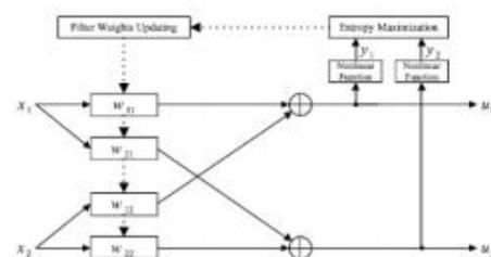
**Fig.2.1 Infomax Based CBSS Division System For Those Two-Source Also Two Sensor. The Event. This System Holds Four Causal Fir Filters  $W_k$  Ij, Also  $U_i$  Will Be Those Divided Indicator**
