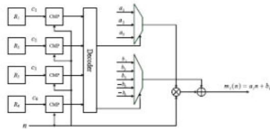
**Fig.3.4 Proposed Scaling Factor Computation Module**
