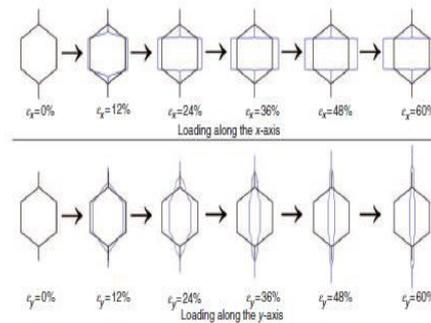
Successive deformations of an individual cell of the core when subjected to increasing loads.
