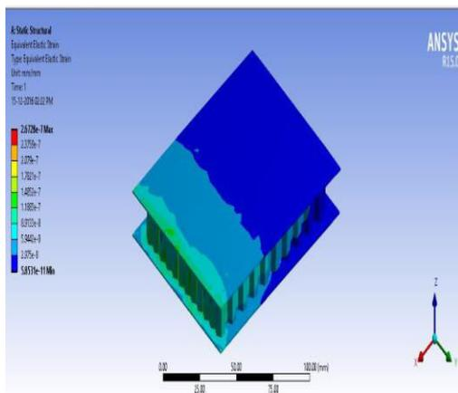
Equivalent elastic strain for steel
