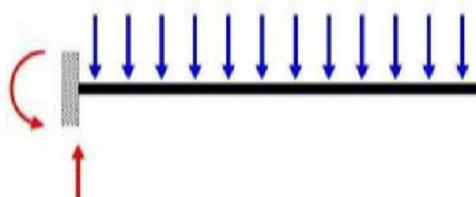
Cantilever beam with UDL
