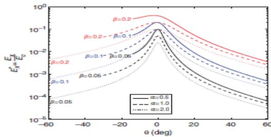
Figure 14. Modulus of cellular core in x-direction.
