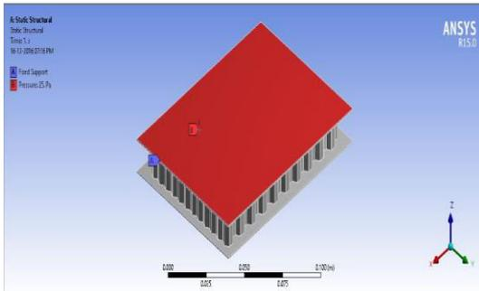
Pressure applying on the panel, by keeping other side DOF as zero
