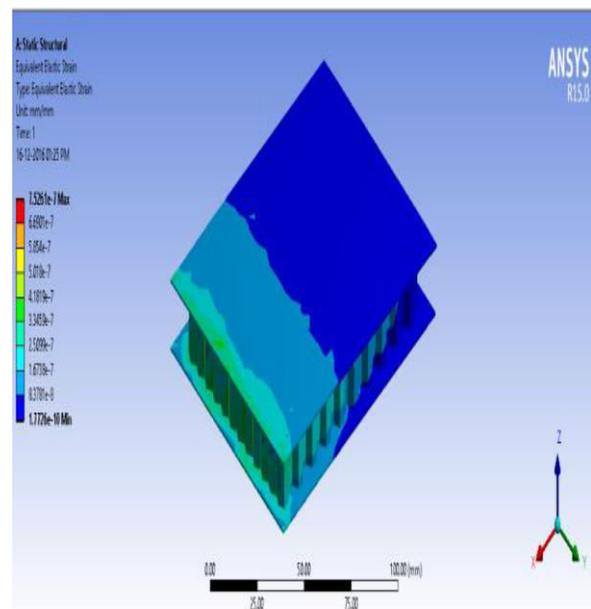
Equivalent elastic strain for aluminium
