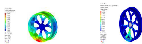
Fig 24: Optimized Model Results Displacement is 0.049m
