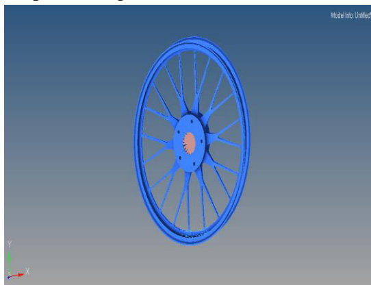
Fig 10: Reference model is imported in to Hyper mesh for preprocessing
