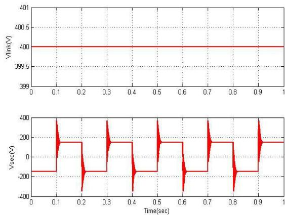
Fig .6:Simulation results of Precharge of the link voltage  $V_{link}$  with  $D = 0.5$  and passive rectifier.  $V_{in} = 30$  V
