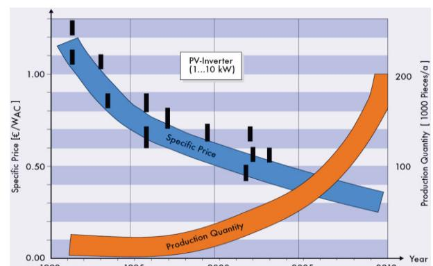
Figure 2: Development and prognoses of specific cost and production quantity for a PV inverter of nominal power between 1 and 10kW during the last two decades.
