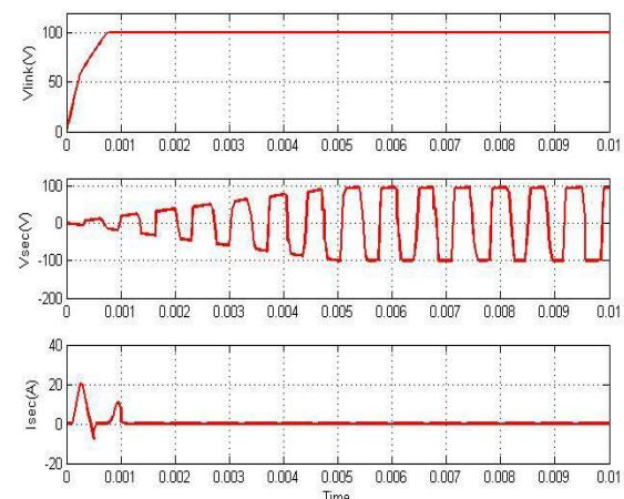
Fig. 8. Simulink results Inrush secondary current and building up of secondary voltage and link voltage for  $D = 0.5$  and input voltage  $V_{in} = 10V$ .
