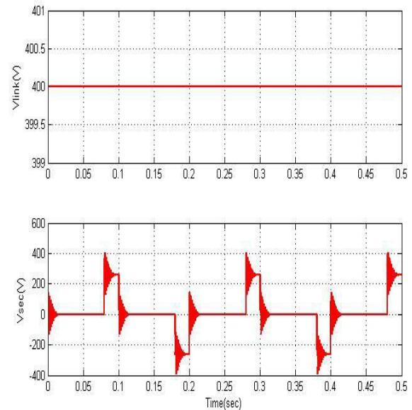
Fig. 10.Simulation results Precharge of the link voltage  $V_{link}$  with  $D = 0.08$  and passive rectifier.
