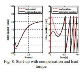
Simulations also show that the system can start up when there is a block torque and in steady state, the compensation has very little effects in rotor speed and position estimation.
