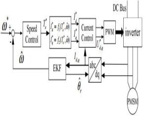
Fig. 1. Block diagram of the sensorless system
