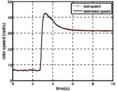
Fig. 9. The estimated and real speeds during acceleration
