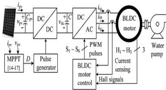
Fig.1. Conventional SPV-fed BLDC motor-driven water pumping system
