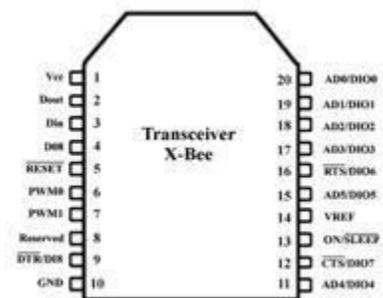
Fig 2: ZIGBEE pin diagram
