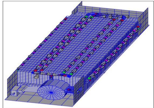
Figure 4.4 Battery pack cooling system with the fluid stream
