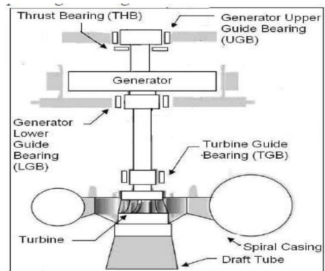
**Figure 1.2. Bearing arrangement of the hydro-electric power generating unit**
