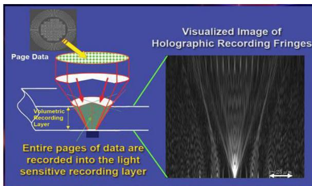
Illustration of what the holographic image looks like as it is being written onto the recording layer.
