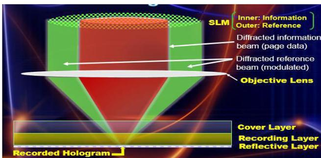
Animation showing the information beam and the data beam of the Holographic laser.
