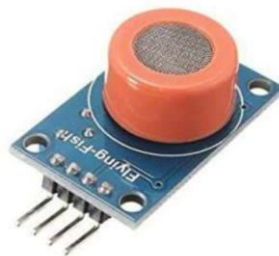
Fig. 4. MQ3 Alcohol sensor
