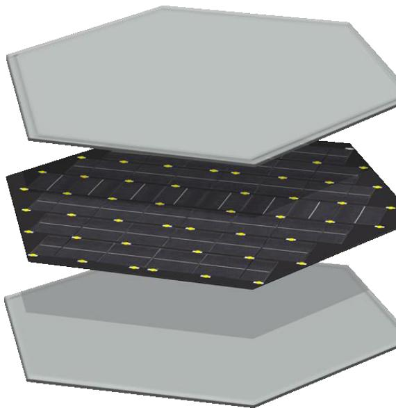
Figure 3. Layers of Solar roadway
