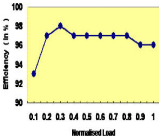
Figure (9): Efficiency of inverter
