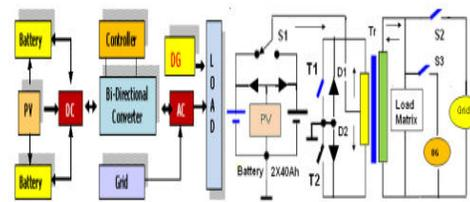
Figure (2): Block and Circuit Model of utility interface Solar Power Converter System
