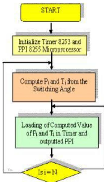
Figure (4): Flow Chart of PWM Pulse Generation Program
