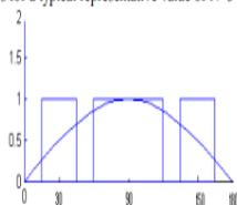
Figure (3): Simulated Direct modulated Sinusoidal PWM pulses for N = 3 in one half cycles (10ms=180 Deg), Frequency = 50 Hz (Scale X = Degree; Y= Pulse Voltage x 5V)
