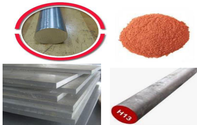
Figure 2: (a): Al-6065 bar (b): Copper powder (c) H13 Material
