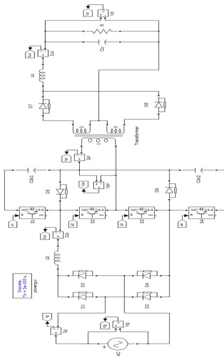
Fig. MATLAB simulation diagramm of proposed three-level single-stage fully integrated PFC ac-dc converter
