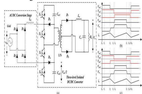
Fig. 2.1 Derivation of the proposed single-stage PFC converter; (a) topology, (b) switching scheme of the conventional three-level dc/dc converter, and (c) modified switching scheme
