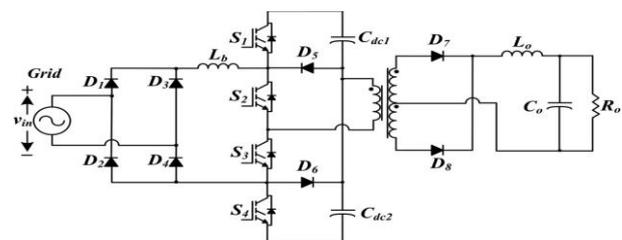
Fig. 1 Proposed three-level single-stage fully integrated PFC ac-dc converter
