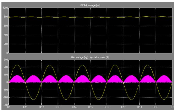
Fig. simulated waveforms: Input voltage, input current, dc-link voltage
