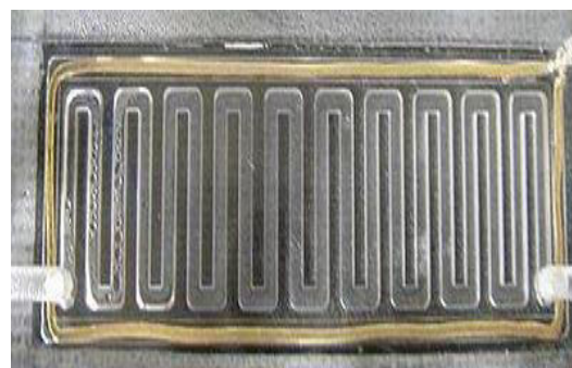
Fig 2.2 Buildup of water delivered by a PEMFC broadcasting live channel divider. The gold wire around the cell guarantees the gathering of electric current.
