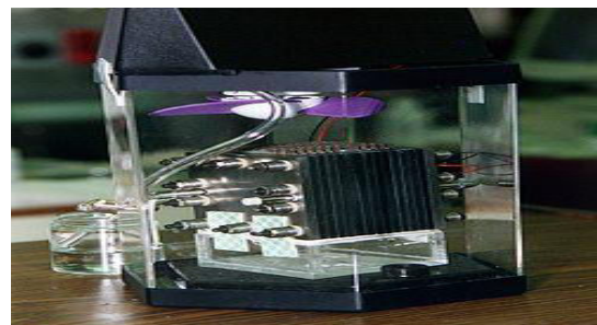
Fig.2.1 Exhibition model of an immediate methanol power module. The genuine energy unit stack is the layered 3D square
