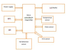
The function working is elucidated as the Arduino will takes the readings of heart beat pulse, body temperature, cough count and fits detection from the respective sensors and orders GSM shield to send an SMS message containing these readings, patient information and the location of the patient which has been taken via GPS shield to the medical expert so that instant remedy can be taken.
