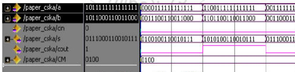
Figure 7: Waveform of Proposed-CSKA
