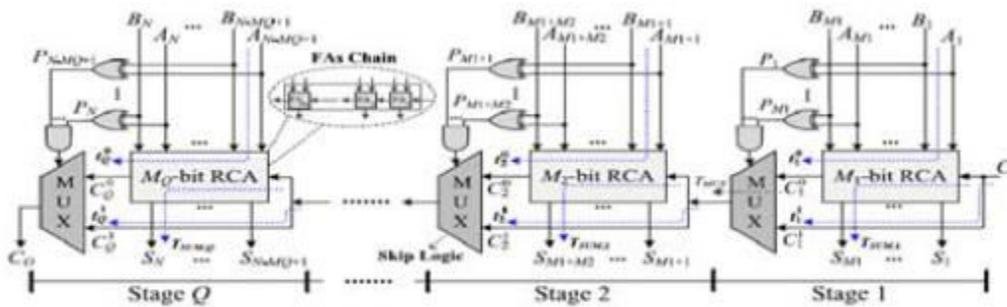
Figure 2: Structure of conventional CSKA
