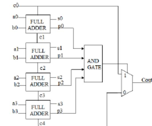
Figure 1: Four bit carry skip adder
