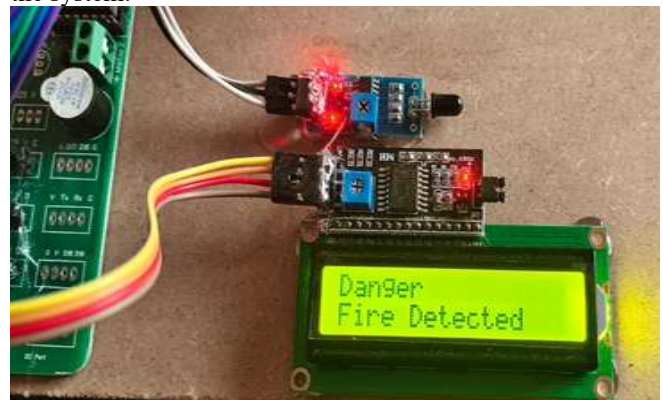
Fig. 4. Flame Detection Indication on LCD
