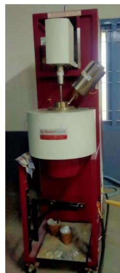
polishing were done. The test component received a 125 kg load for 15 seconds, and the diameter of the impression was
