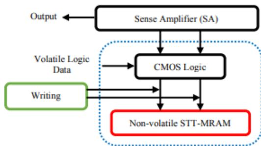
**Fig.3.3. Structure of a MTJ based circuit.**
