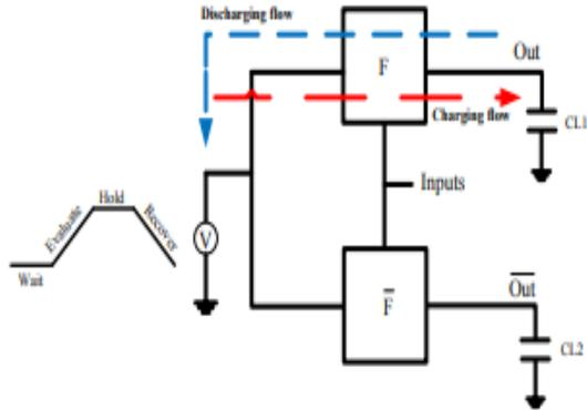
**Fig.3.2. Circuit representing adiabatic charging/discharging.**
