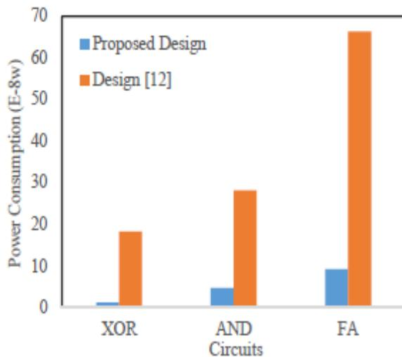
**Fig.3.6. Power consumption of the proposed designs and designs.**
