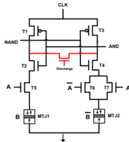
**Fig.3.4. Proposed adiabatic hybrid MTJ/CMOS AND/NAND.**
