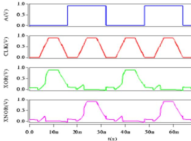
**Fig.3.5. Transient response of the proposed adiabatic hybrid MTJ/CMOS.**
