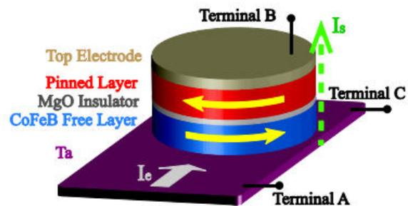
**Fig.3.1. Three-terminal device based on the giant spin Hall effect.**
