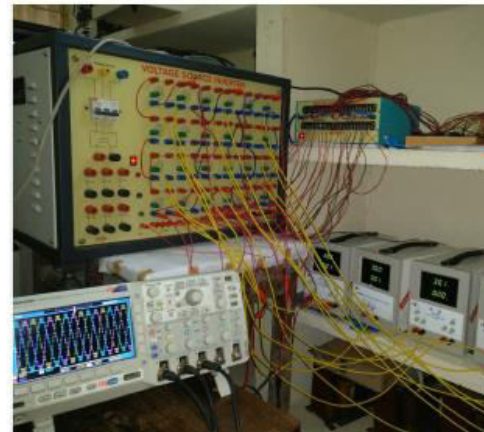
Fig. 7 Photograph of the experimental set-up for realising 13-level asymmetrical switched dc source inverter
