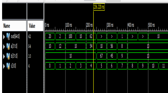
Fig.3.4. ALU Simulation circuit.
