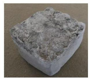
Fig.2: Aluminium 6351 Precursor obtained after solidification
