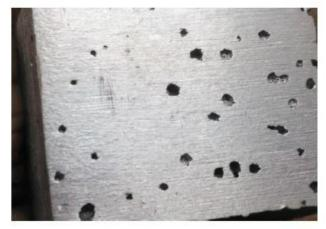
Fig.3: Aluminium 6351 foam obtained after annealing
