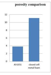
Fig.6: variation of porosity in Al 6351 parent metal and developed foam
