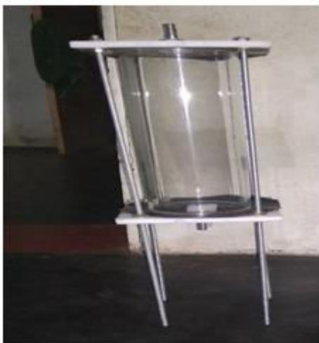
Figure 3. Electrolyser solution tank capacity of 2.5liters
