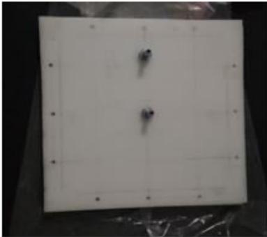
Figure: 2.1 (b) Nylon plates clamping together with S.S bolts.
