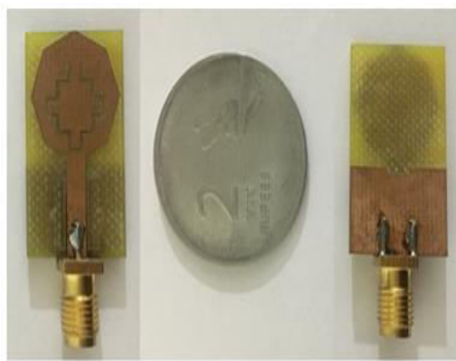
Figure-10. Fabricated antenna
