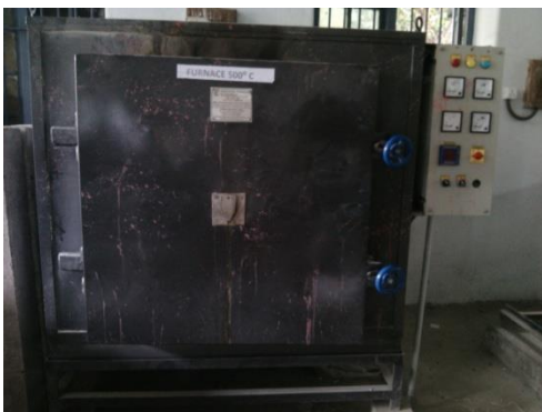
Furnace used for heat curing
