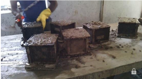
Compaction of GPC cubes on vibrating table
