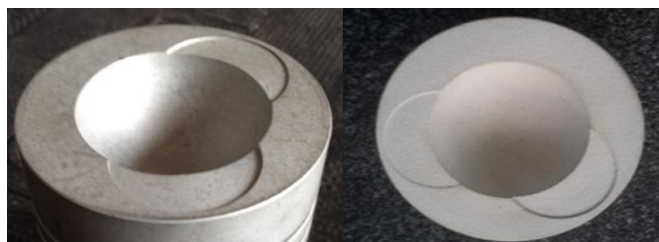
Fig 3. Uncoated baseline engine piston (left) and YSZ coated piston (right).
