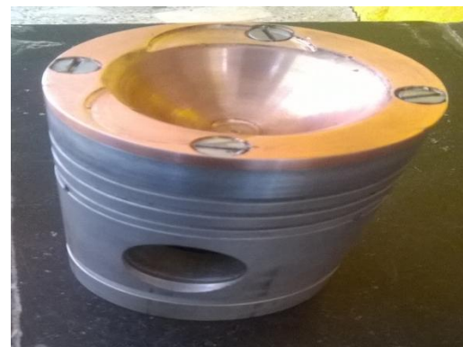
Figure 3: Semi-Adiabatic Air-Gap Copper Crown Piston
