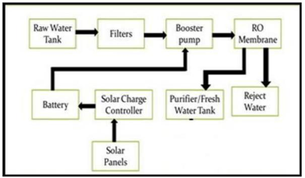
created by booster pump to carry out reverse osmosis process. The microcontroller keeps watch to level of the water tank and prevents it from the overflow. By using this process, we obtain pure water in the water tank.[5]
