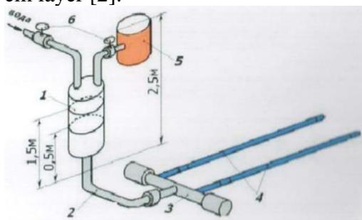
1 water level stable container; 2 water intake plastic pipe; 3 distribution pipe; 4-drop polyethylene pipe; 5 container of mineral and organic fertilizers; 6 taps. [3,4,9].
