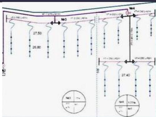
Figure 1. Schematic diagram of a low-pressure drip irrigation system in an experimental field
